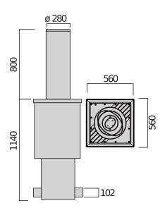
Automatic hydraulic anti-terrorism bollard, tested and certified (crash-tested) by independent body in accordance with standards IWA14-1:2013 and PAS 68 (equivalent to American standards K12 and K4), with independent hydraulic control unit. Suitable for the protection of sensitive sites. Independent side hydraulic pump for each bollard: in case of a control unit failure the other bollards remain functional, whereas maintenance operations are facilitated.
