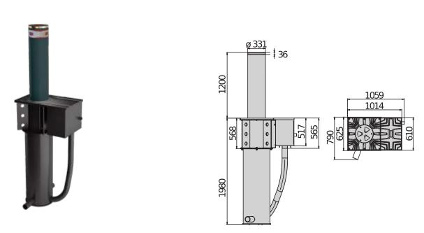
Automatic hydraulic anti-terrorism bollard, tested and certified (crash-tested) by independent body in accordance with standards IWA14-1:2013 and PAS 68 (equivalent to American standards K12 and K4), with independent hydraulic control unit. Suitable for the protection of sensitive sites. Independent side hydraulic pump for each bollard: in case of a control unit failure the other bollards remain functional, whereas maintenance operations are facilitated.
