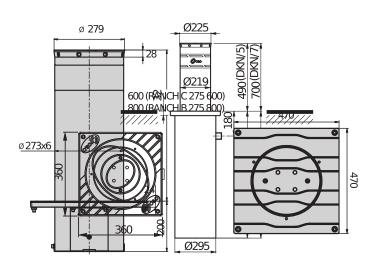
Fixed bollards used for preventing access for long periods. Bolted to the ground, their purpose is to block an access point or a road. They can integrate the use of automatic or semi-automatic bollards.
