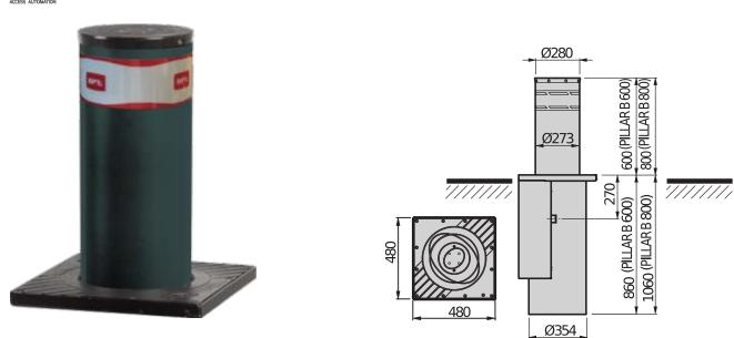
Anti-terrorist hydraulic bollard with incorporated hydraulic control unit. Suitable for protecting sensitive sites, thanks to the special "SD" version, which keeps the shaft raised in case of a power failure and with public installations where, in the standard version, the shaft lowers automatically with no power.
