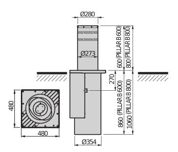
Anti-terrorist hydraulic bollard with incorporated hydraulic control unit. Suitable for protecting sensitive sites, thanks to the special "SD" version, which keeps the shaft raised in case of a power failure and with public installations where, in the standard version, the shaft lowers automatically with no power.
