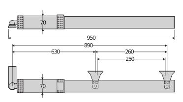
Extremely compact and sturdy hydraulic operators suitable for residential and small condominium use. Capable of automating swing gate leaves up to 2.5 metres wide and weighing up to 200 kg. Available in both reversible and irreversible versions. Maximum precision in force control guaranteed by by-pass valves.
