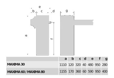
Range of professional 230 Vac electro-mechanical barriers for frequent use, designed to work under a great variety of conditions including large car parks, motorway toll gates with frequent reversing, industrial installations. Mechanical movement with crank to make the bar operate smoothly and harmoniously, also managing slowdowns in opening and closing.
