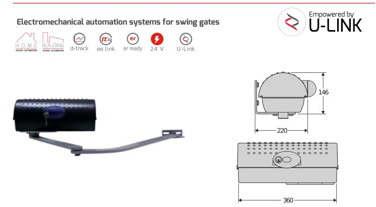
Range of irreversible electro-mechanical 24 v operators for swing gates up to 250 kg in weight and up to 2.5 m in length. Ideal for installation on large-size pillars thanks to its articulated levers that allow opening up to 125°.
