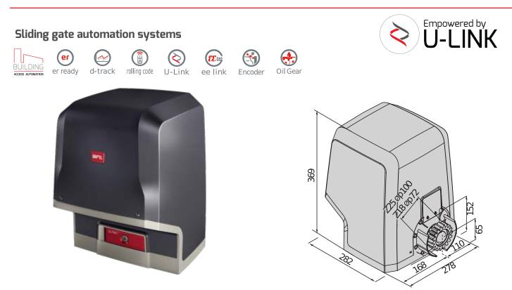
230V sliding gate operators for very intensive use, extremely sturdy and high-performance thanks to oil bath transmission. Control of torque via D-track technology and absolute encoder for maximum precision of movement. Control unit arranged for communication with U-link protocol and with tamper-proof function.
