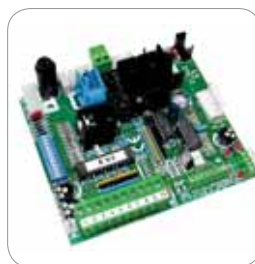
Incorporated electronic control board ELPRO 63, pre-set to take the plug-in radio receiver
