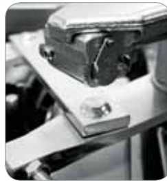
Detail of the emergency manual release
