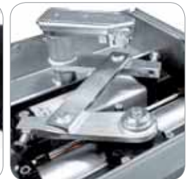
Detail of the motor-pump and jack
