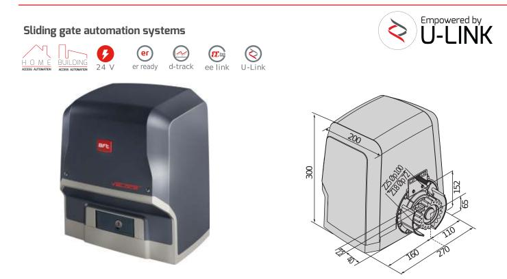
Fast-action 24V operator for intensive use for sliding gates up to 500kg. Speed without load 25 m/min. Torque control thanks to D-Track technology. Control unit for communication with U-Link protocol. Operator with electromagnetic limit switch. The ideal solution for situations which require fast operating speeds, reduced waiting times and high levels of security.
