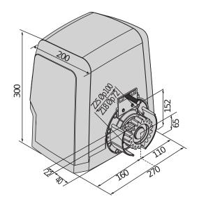
Range of 24V sliding gate operators for intensive use with leaves up to 1500 kg, maximum leaf speed 12 m/min
